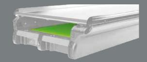
The space dedicated to the housing of immobilization systems (Backboard or pick up stretcher) is equipped with stabilizer; a highly innovative system that ensures firm anchoring and is silent during transport.
