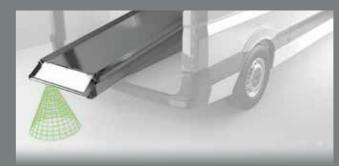
the ground thanks to a patented sensor. Based on the data received, it will self adjust to the ideal height for unloading so the stretcher legs will always open up to a safe position.
